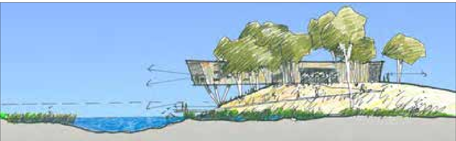
SECTION 1 - Visitor Centre elevation above Jerrabomberra Creek (100yr flood). Walkways engage with the Wetlands at the lower level.
